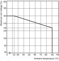
Note. The maximum coil voltage refers to the maximum voltage in a varying range of operating power voltage, not a continuous voltage.
